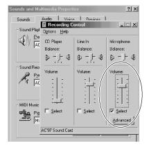
**5.** In the Microphone group, check the **Select** box to enable the microphone input, and set the microphone volume to about 60% of the full scale.
